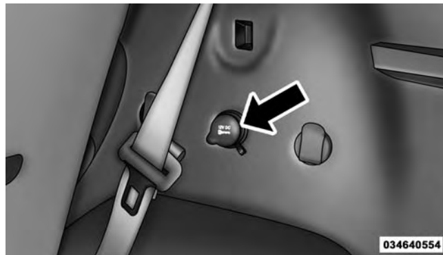
Rear Cargo Power Outlet
