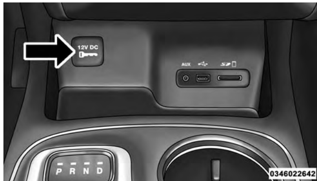
Front Power Outlet
