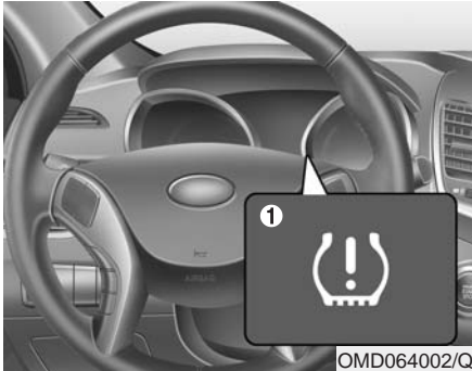
(1) Low Tire Pressure Telltale/ TPMS Malfunction Indicator
