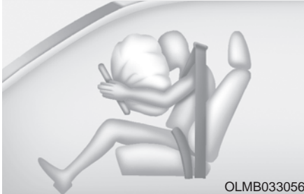
■ Passenger's front air bag
