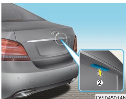
(2) Power Trunk Open button
