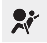
SRS warning light
