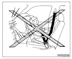
Even with the NISSAN Advanced Air Bag System, never install a rear-facing child restraint in the front seat. An inflating front air bag could seriously injure or kill your child. For additional information, refer to "Child restraints" in this section.
