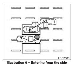
Illustration 6:If the driver activates the turn signal while another vehicle is in the detection zone. then the system chimes (twice) and the side indicator light flashes.
