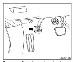
**To engage:** Firmly depress the parking brake.
