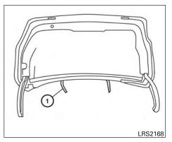
To fold down the driver side of the rear seat, open the trunk and pull on the strap ①.
