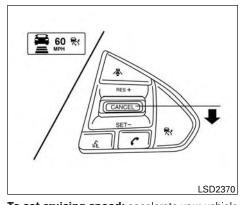
To set cruising speed: accelerate your vehicle to the desired speed, push the SET- switch and release it. The ICC system set indicator (green), vehicle ahead detection indicator, set distance indicator and set vehicle speed indicator (B) will come on. Take your foot off the accelerator pedal. Your vehicle will maintain the set speed.
