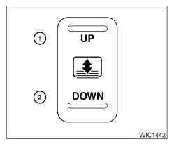
The rear sun shade operates when the ignition switch is in the ACC or ON position.
