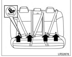
**LATCH** system lower anchor locations LATCH (Lower Anchors and Tethers for CHildren) SYSTEM
