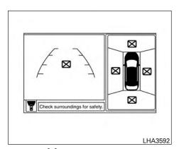
When the "[X]" icon is displayed on the screen, the camera image may be receiving temporary electronic disturbances from surrounding devices. This will not hinder normal driving operation but the system should be inspected by a NISSAN dealer if it occurs frequently.
