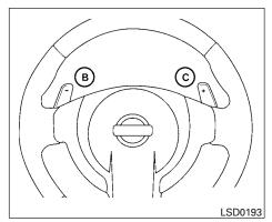
manually. Shift ranges can also be selected using the shift paddles (if so equipped) on the steering wheel (B) and (C). In the manual shift mode, the shift range is displayed on the position indicator in the meter. When shifting the shift lever to the manual shift gate, the position indicator displays 1 (first) up to 7 (seventh) depending on vehicle speed.
