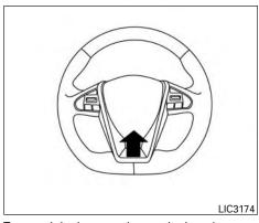
To sound the horn, push near the horn icons on the steering wheel.
