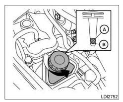
Check the fluid level in the reservoir.
