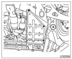
4. Remove clips **(B)** from the under-engine protector.
