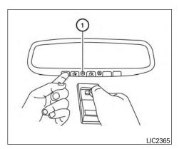
2. Using both hands, simultaneously press and hold the desired HomeLink® button and handheld transmitter button. DO NOT release until the HomeLink® indicator light ① flashes slowly and then rapidly. When the indicator light ① flashes rapidly, both buttons may be released. (The rapid flashing indicates successful programming.)
