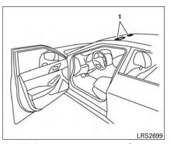
1. SRS Air Bag Warning Labels (located on the sun visors)
