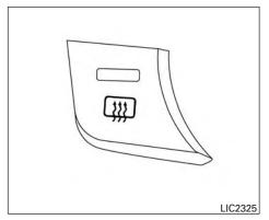
To defrost the rear window glass and outside mirror (if so equipped), start the engine and push the rear window defroster switch on. The rear window defroster indicator light on the switch comes on. Push the switch again to turn the defroster off.
