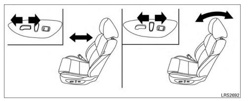
The reclining feature allows adjustment of the seatback for occupants of different sizes for added comfort and to help obtain proper seat belt fit. For additional information, refer to "Precautions on seat belt usage" in this section. Also, the seatback can be reclined to allow occupants to rest when the vehicle is stopped and the shift lever is in P (Park).
