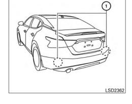
The RCTA system uses radar sensors 1 installed on both sides near the rear bumper to detect an approaching vehicle.
