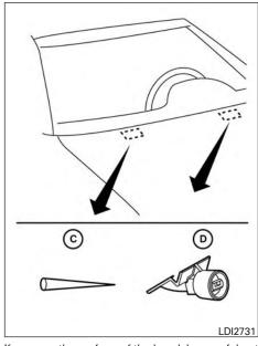
If you wax the surface of the hood, be careful not to let wax get into the washer nozzle (D). This may cause clogging or improper windshield-washer operation. If wax gets into the nozzle, remove it with a needle or small pin (C).
