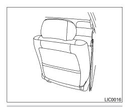
Do not place heavy loads heavier than 2.2 lbs. (1 kg) on the seatback, head restraint/headrest or in the seatback pocket.
