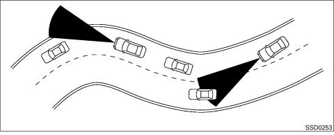
When driving on some roads, such as winding, hilly, curved, narrow roads, or roads which are under construction, the radar sensor may detect vehicles in a different lane, or may temporarily not detect a vehicle traveling ahead. This may cause the ICC system to decelerate or accelerate the vehicle.
