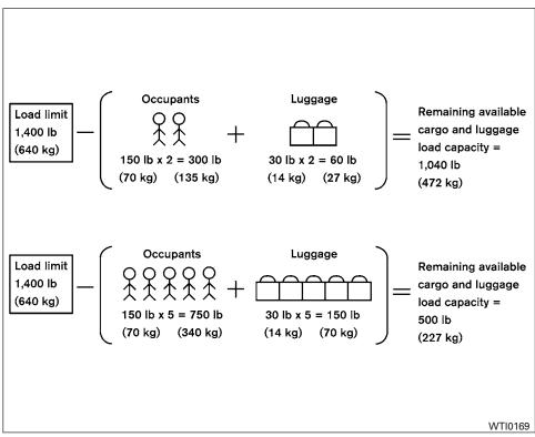
Steps for determining correct load limit
