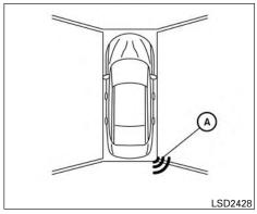
When the corner of the vehicle moves closer to an object, the corner sonar indicator (A) appears.
