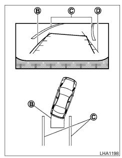
Slowly back up the vehicle adjusting the steering wheel so that the predicted course lines
