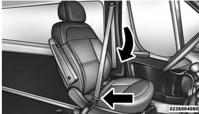
Inserting Latch Plate Into Buckle
