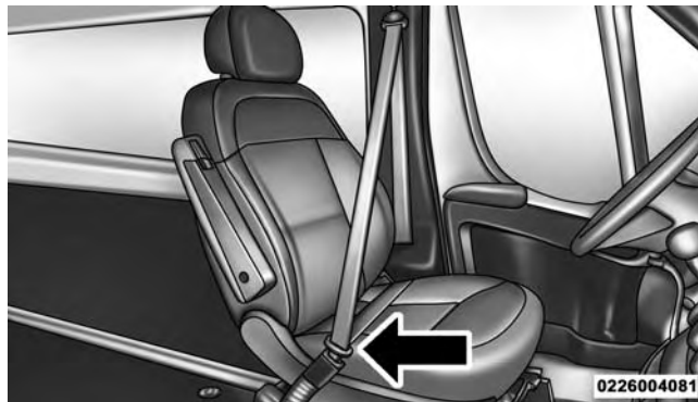
Pulling Out The Latch Plate
