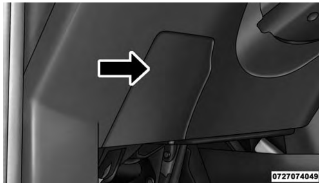
Fuse Panel Cover
