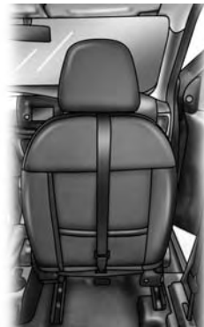
Tether Strap Installation
