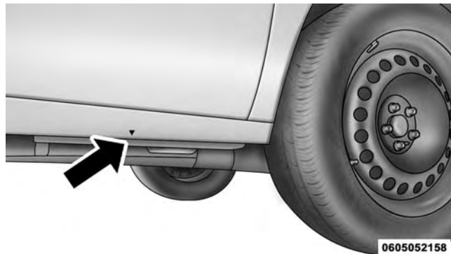
Front Jacking Location
