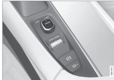
Start knob in the tunnel console
