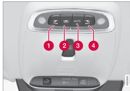
Controls in the ceiling console for front reading lights and courtesy lighting
