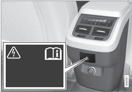
120-volt socket in the tunnel console for the second row of seats
