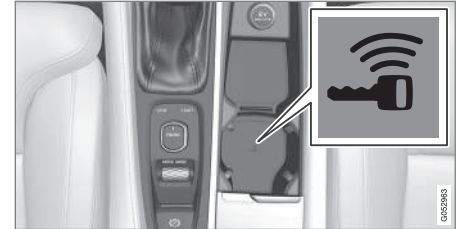
Back-up reader in the tunnel console
