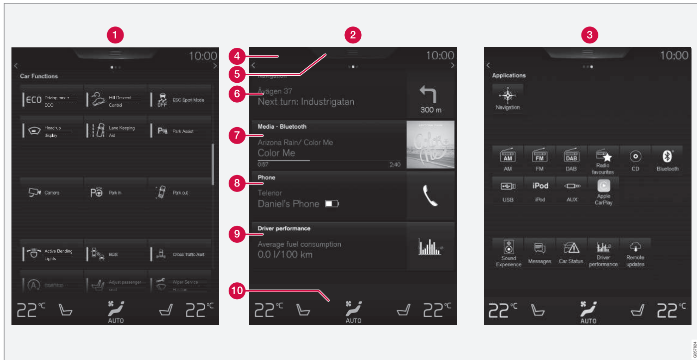
Three of the center display's basic views. Swipe to the right/left to access the Function/App view (generic illustration)
