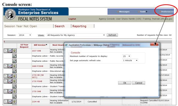
The pagination function allows users to select the number of rows displayed on each page. The refresh rate function allows users to set the rate at which the Console screen will refresh with new information. The system can display a maximum number of 100 bills on a single page. Please note that by choosing a larger number of bills to display, there is an associated increase in processing time to fill/refresh the page.
