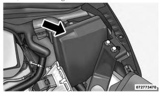
The ID number of the electrical component corresponding to each fuse can be found on the back of the cover.
