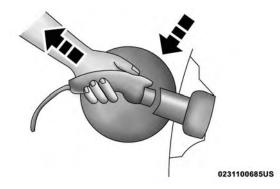
Removing The Charge Connector From The Vehicle **Charge Inlet**
