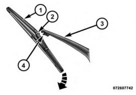
Removing The Wiper Blade
