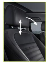
Tilt the head restraint forward for additional comfort by gently pulling the top of the head restraint. Once it is in the forward-most position, tilting it forward again releases it to the upright position.
