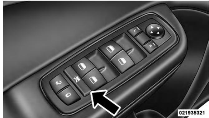
Window Lockout Switch
