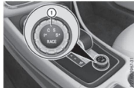
► Turn DYNAMIC SELECT controller ① as many times as necessary until the desired drive program is selected. The selected drive program appears in the multifunction display. After five seconds the display goes out and the status icon of the selected drive program appears. The drive program indicator on DYNAMIC SELECT controller ① lights up in red.
