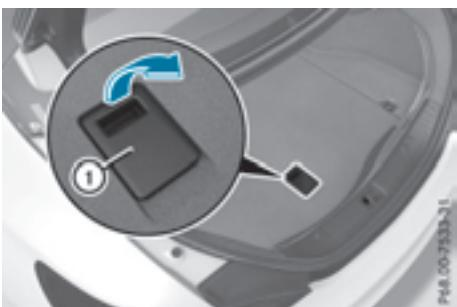
Under the trunk floor you can find a bracket for TIREFIT and the vehicle tool kit, etc.
