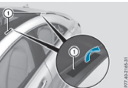
► Open and fold the covers ① upwards carefully in the direction of the arrow.
