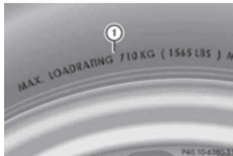
Maximum tire load ① is the maximum permissible weight for which the tire is approved. Do not overload the tires by exceeding the specified load limit. The maximum permissible load can be found on the vehicle's Tire and Loading Information placard on the B-pillar on the driver's side (▷ page 292).
