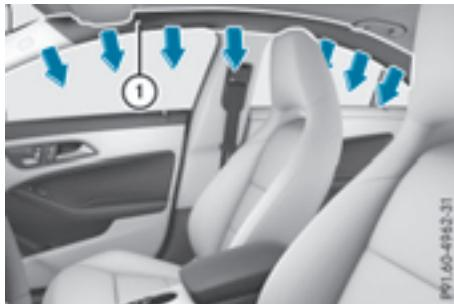
Window curtain air bags ① are integrated into the side of the roof frame and deployed in the area from the A-pillar to the C-pillar.
