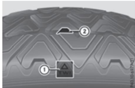
Marking ① shows where bar indicator ② for tread wear is integrated into the tire tread.
