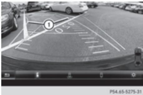
① Yellow guide line for the vehicle width including the exterior mirrors, for current steering wheel angle (dynamic)
