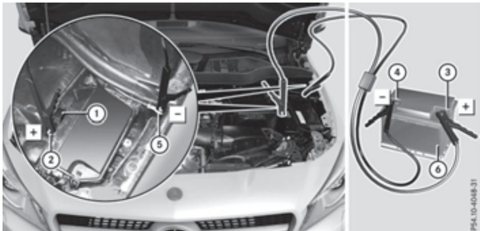
Position number ⑥ identifies the charged battery of the other vehicle or an equivalent jump-starting device.
