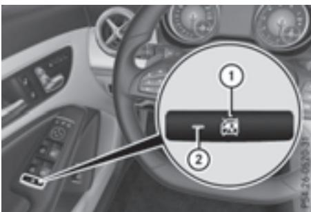
▶ **To activate/deactivate:** press button ①. If indicator lamp ② is lit, operation of the rear side windows is disabled. Operation is only possible using the switches in the driver's door. If indicator lamp ② is off, operation is possible using the switches in the rear compartment.
