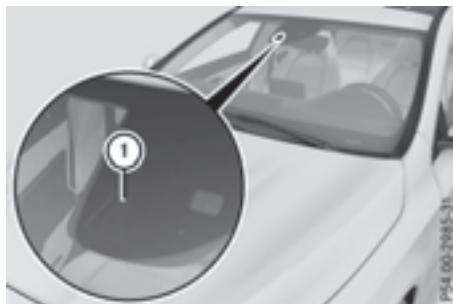
Lane Keeping Assist monitors the area in front of your vehicle by means of multifunction camera ① which is attached behind the top of the windshield. Active Lane Keeping Assist detects lane markings on the road and can warn you before you leave your lane unintentionally.
