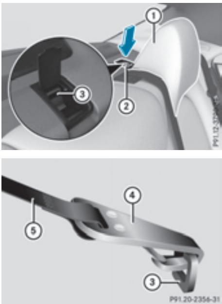
The Top Tether anchorage points are installed in the rear compartment behind the head restraints on the parcel shelf.
