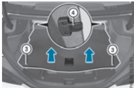
► **To insert:** place the trunk floor at the bottom in the center.
