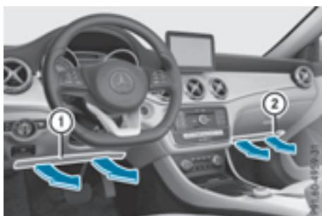
Driver's knee bag (1) deploys under the steering column and front-passenger knee bag (2) under the glove box. The driver's and front-passenger knee bags are triggered together with the front air bags.
