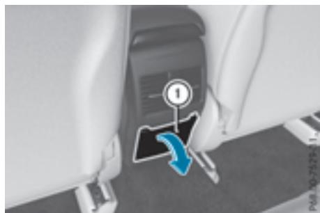
► **To open:** pull down the top of stowage compartment ① by the edge of the handle.
