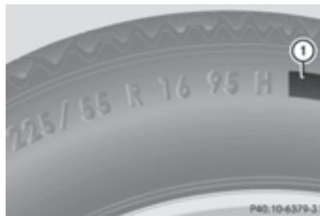
In addition to the load-bearing index, load index ① may be imprinted after the letters that identify speed rating on the sidewall of the tire. Speed rating (▷ page 296).
