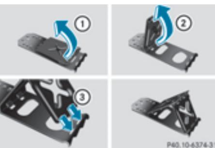
If your vehicle is equipped with a wheel chock, it can be found in the tire-change tool kit (▷ page 266).
