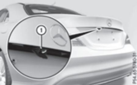
Rear view camera ① is an optical parking and maneuvering aid. It shows the area behind your vehicle with guide lines in the multimedia system display.
