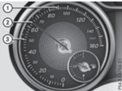
When Distance Pilot DISTRONIC is activated and there are no vehicles detected in front, one or two segments ② in the speed range set light up.
