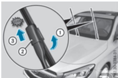
▶ Hold on to the wiper arm with one hand. With the other hand, turn wiper blade in direction of arrow ① away from the wiper arm as far as it will go.
