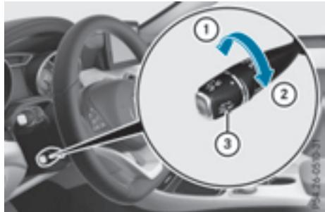
► **To increase:** turn control ③ in direction ②. Distance Pilot DISTRONIC then maintains a greater distance between your vehicle and the vehicle in front.
