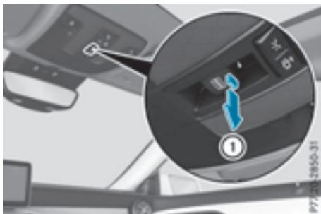
Reset the panorama roof with power tilt/sliding panel or the roller sunblind, if the panorama roof with power tilt/sliding panel or the roller sunblind does not move smoothly.
