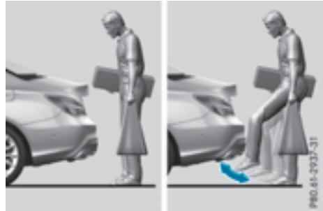
► **To open:** kick into sensor detection range ① below the bumper with your foot.
