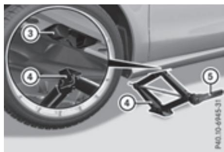
► Take ratchet wrench ⑤ out of the vehicle tool kit and place it on the hexagon nut of jack ④ so that the letters **AUF** are visible.
