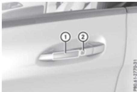
► **To unlock the vehicle:** touch the inner surface of the door handle.
