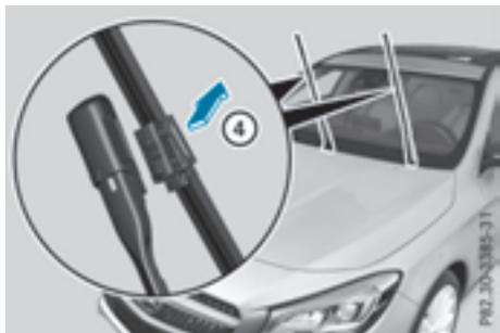
▶ Remove the wiper blade in the direction of arrow ④ away from the wiper arm.
