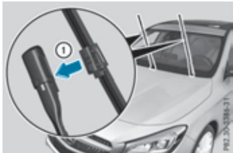
▶ Insert the new wiper blade into the wiper arm in the direction of arrow ①.
