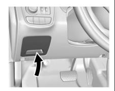
The instrument panel fuse block is on the underside of the driver side instrument panel.
