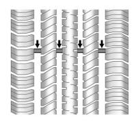
Treadwear indicators are one way to tell when it is time for new tires. Treadwear indicators appear when the tires have only 1.6 mm (1/16 in)
