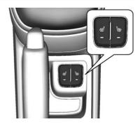
If equipped, the buttons are on the center console. To operate, the engine must be running.
