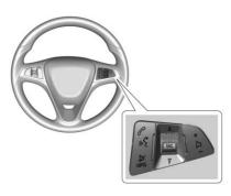
For vehicles with audio steering wheel controls, some audio controls can be adjusted at the steering wheel.
