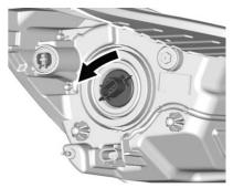
Remove the headlamp bulb socket.
