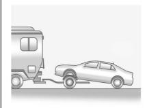
To tow the vehicle with the two rear wheels on the ground and the front wheels on a dolly:
