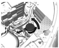
Remove the washer funnel by turning it counterclockwise and pulling it straight out.
