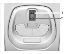
Vent/Open: Press and hold (1) to vent. Press and hold (1) again to open the sunroof. Release the switch to stop movement. The sunshade automatically opens with the sunroof, but must be closed manually.
