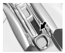
3. Place the new transmitter into the transmitter pocket.
