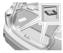
The cargo tie-downs can be used to secure small loads.
