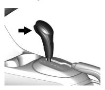
**P**: This position locks the front wheels. Select P (Park) only when the vehicle is stationary and the parking brake is applied.
