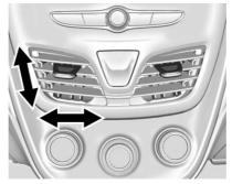
Move the slats to change the direction of the airflow. The center air vent does not close completely.
