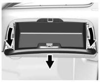
Open the glove box completely and loosen the bolts on the outboard side.
