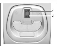
Vent/Open: Press and hold (1) to vent. Press and hold (1) again to open the sunroof. Release the switch to stop movement. The sunshade automatically opens with the sunroof, but must be closed manually.
