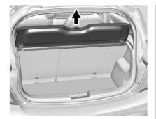
To remove, pull the cargo cover upward.
