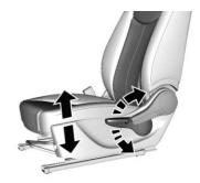
If available, move the lever up or down to manually raise or lower the seat.
