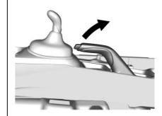
To release the parking brake, hold the brake pedal down. Pull the parking brake lever up until you can press the release button. Hold the release button in as you move the brake lever all the way down.
