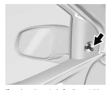
If equipped, controls for the outside manual mirror are next to each mirror. Adjust to see a little of the side of the vehicle.
