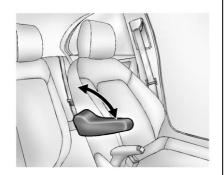
There is an armrest on the inboard side of the driver seat. To raise or lower the armrest, push up or pull down on the armrest.
