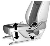
If equipped, move the lever up or down to manually raise or lower the seat.
