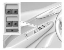
Press the switch down to open the window. Pull the switch up to close it.
