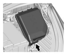
The engine compartment fuse block is on the driver side of the vehicle, near the battery.
