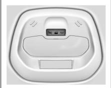
The dome lamp controls are in the headliner above the front seats.
