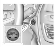
The vehicle may be equipped with an electronic keyless ignition with pushbutton start.
