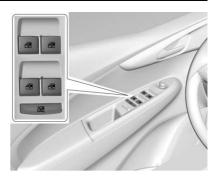
The windows work when the vehicle is in ON/RUN, ACC/ACCESSORY, or Retained Accessory Power (RAP). See Retained Accessory Power (RAP) ⇒ 182.
