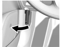
Pull the hood release handle inside the vehicle. It is on the lower left side of the instrument panel.
