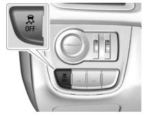
The button for TCS and StabiliTrak is on the lower instrument panel to the left of the steering wheel.
