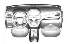
The driver knee airbag is below the steering column. The front outboard passenger knee airbag is below the glove box.
