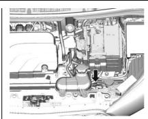
2. Open the hood and unwrap the electrical cord. The cord is located in the driver side of the engine compartment, near the engine coolant surge tank. It is shipped from the factory with a tie holding it in place. Use care in removing the tie so that the cord is not damaged.
