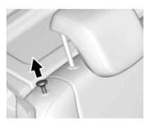
4. Pull up the release knob on the top of the seatback.
