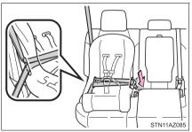
3 Fully extend the shoulder belt and allow it to retract to put it in lock mode. In lock mode, the belt cannot be extended.
