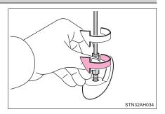
2 Using the wrench, tighten the antenna an additional 1/8th turn (20 to 45 degrees) to secure it in place.
