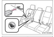
Seat belts equipped with a child restraint locking mechanism (ALR/ELR belts except driver's seat belt) (→P. 34)
