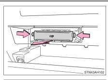
6 Pull the filter out of the filter outlet.
