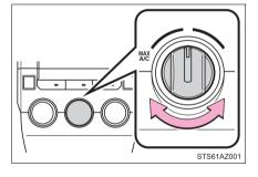
The air conditioning will automatically turn on and the air intake selector will be set to recirculated air mode.
