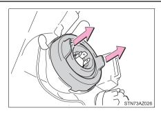
4 Release the bulb retaining spring.
