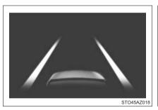
Indicates that the system is recognizing white (yellow) lines. When the vehicle departs from its lane, the white line displayed on the side the vehicle departs from flashes orange.
