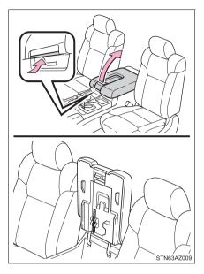
▶ Front bench type seat Pull the lever up and fold down the seatback
