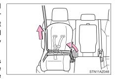
5 If the child restraint has a top tether strap, the top tether strap should be latched onto the top tether strap anchor. (→P. 67, 70)
