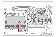
Under the instrument panel Remove the cover.
