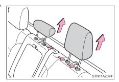
Route the top tether strap through the anchor strap belt as shown in the illustration.
