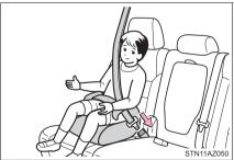
Check that the shoulder belt is correctly positioned over the child's shoulder and that the lap belt is as low as possible.  $(\rightarrow P. 32)$
