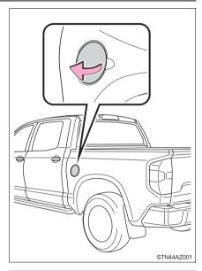
2 Turn the fuel tank cap slowly open, and hang the fuel tank cap on the back of the fuel filler door.
