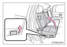
2 On vehicles with storage box, turn the knob to the "OPEN" direction and remove the lid.
