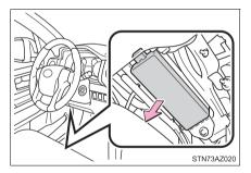
Remove the fuse with the pullout tool.
