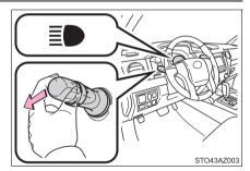
2 Press the Automatic High Beam switch.
