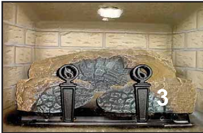
LOG #3 (SRV2032-703): Position log #3 by locating its slot over the tab on right front of the burner such that left end of log contacts log tab near the center of the burner.
