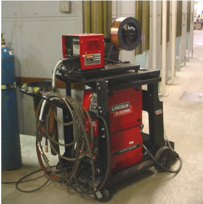
LN7 and Cobramatic wire feeders mated to the Invertec V350 Pro Power source.
