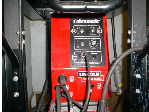
Cobramatic Wire feeder –A Push Pull wire feeder system
