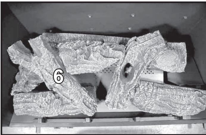
LOG #6 (SRV349-706): Position the "Y" end of log #6 into the cutout on log #4 and its opposite end into the groove on log #2.
