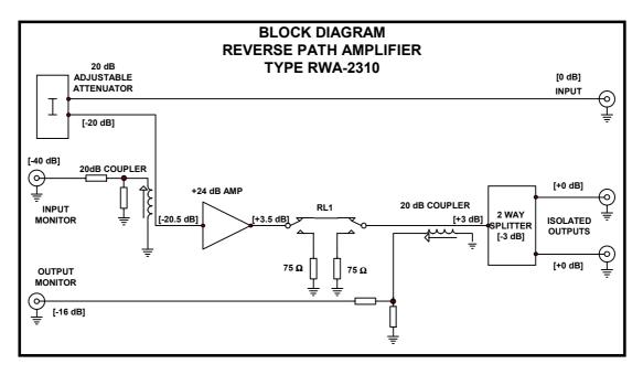
The block diagram for the signal path shows the basic layout of the amplifier and its inputs and outputs. The figures in square brackets indicate the approximate signal levels at various points in the circuit when the amplifier is set to unity gain.
