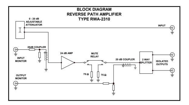
The RWA-2310 has been designed to provide amplification of signals in the reverse path of cable TV distribution systems.
