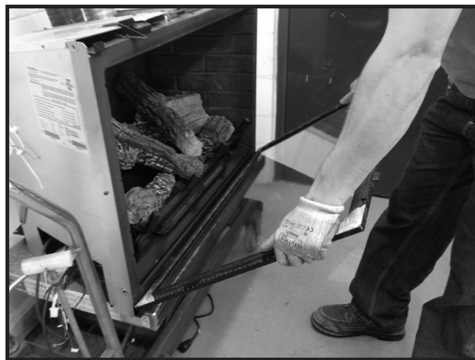
Figure 11.4 Tilt Glass Down and Lift Up to Disengage Bottom Latch
