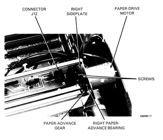
Figure B-9. Paper-Advance Stepping Motor Installation
