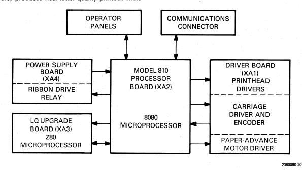
Figure D-1. Simplified Block Diagram of the Model 810LQ Printer
