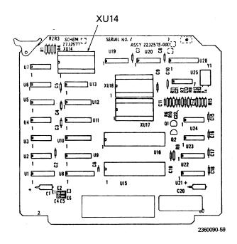
Figure B-7. Location of Socket XU14 on the LQ Upgrade Board
