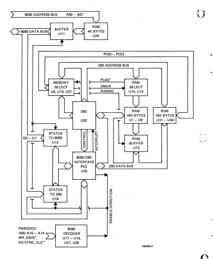
Figure D-2. Simplified First-Generation LQ Upgrade Board Logic Diagram
