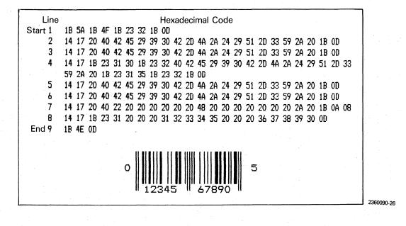
Figure 5-3. Bar-Code Printing Example
