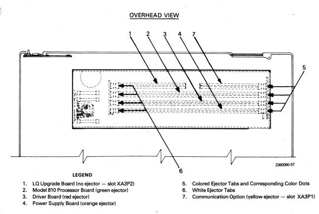
Figure B-5. Location of Printed Wiring Boards - Half-Sized LQ Upgrade Board
