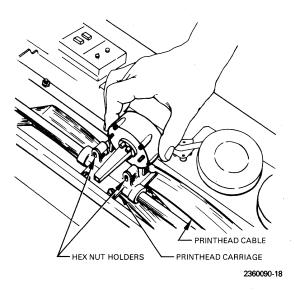
Figure B-10. Printhead Removal and Installation
