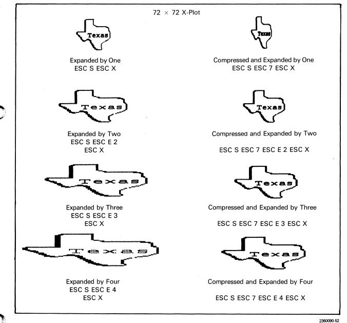
Figure 8-15. Six-Bit, X-Plot Printing Examples
