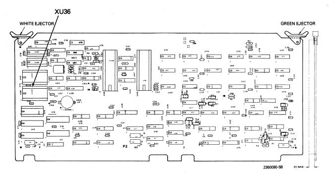
Figure B-6. Location of Socket XU36 on the Model 810 Processor Board
