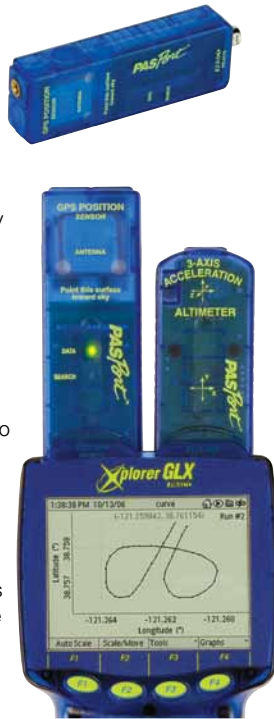
Car acceleration was measured with an Acceleration Sensor, and position and velocity were measured with the GPS Position sensor, then plotted on an aerial photo in My World software. The size of the plotted data point indicates the speed of the car, and the data is color coded to indicate the car's centripetal acceleration.
