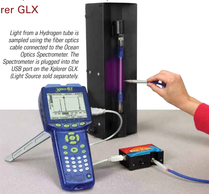
Light from a Hydrogen tube is sampled using the fiber optics cable connected to the Ocean Optics Spectrometer. The Spectrometer is plugged into the USB port on the Xplorer GLX.
