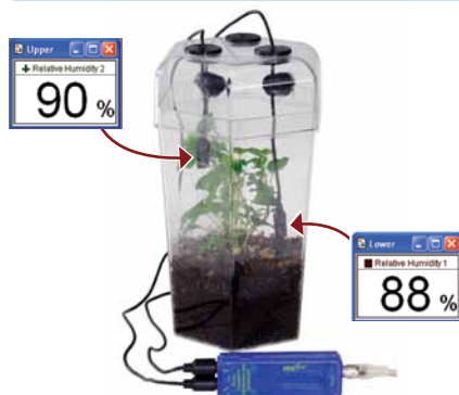
PS-2156 shown in use measuring the difference in relative humidity between foliage and open area in EcoZone™ System ME-6668 (page 61).
