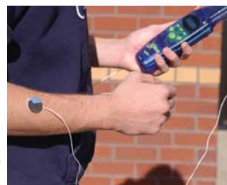
Adhesive patches hold the Temperature Probe in place.
