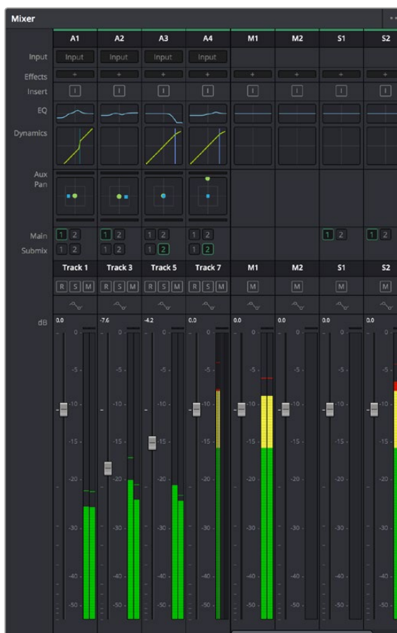
The audio mixer, with channel strips corresponding to the tracks in the timeline
