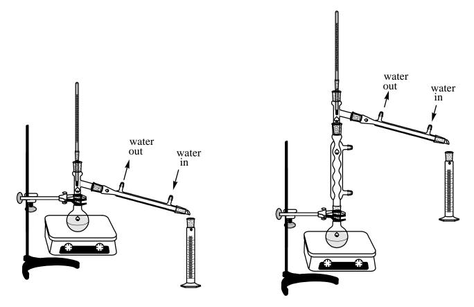
Fig. 3 - The apparatus used in simple distillation
