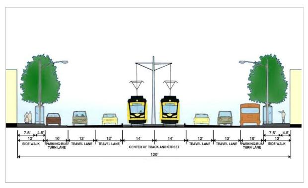
FIGURE 2-9 UNIVERSITY AVENUE TYPICAL CROSS SECTION
