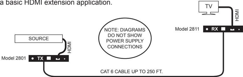
In this configuration, HDMI cables connect the source and display equipment to the respective 2801 Transmitter and 2811 Receiver. A Cat 5 or 6 UTP cable connects the 2801 to the 2811. Properly terminated Cat 6 cables will result in the longest possible range. Terminate the cables to either the EIA 568A or 568B standard for best performance. Correct pairing is vital, and should always be checked with a network cable tester. The DIP switches on the 2801 and 2811 should all be in the DOWN position.
