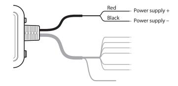
Figure 12 Connecting the power supply
