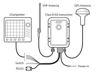
Figure 4 Typical installation configuration
