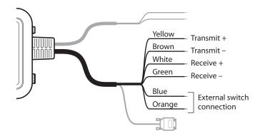
Figure 10 Connecting an external switch
