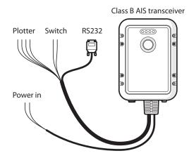
Figure 3 Electrical connections to the Mariner X2
