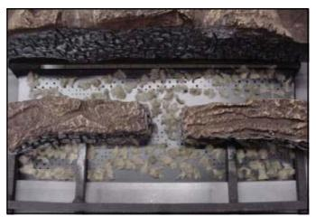
Figure 40. Placement of the Ember Material
