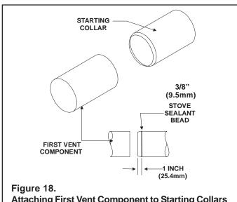
Attaching First Vent Component to Starting Collars
