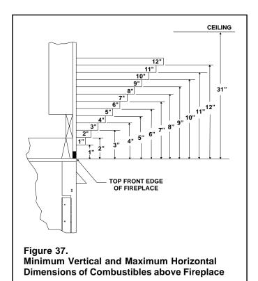
CAUTION: IF JOINTS BETWEEN THE FINISHED WALLS AND THE FIREPLACE SURROUND (TOP AND SIDES) ARE SEALED, A 300° F. MINIMUM SEALANT MATE-RIAL MUST BE USED. THESE JOINTS ARE NOT RE-QUIRED TO BE SEALED. ONLY NON-COMBUSTIBLE MATERIAL (USING 300° F. MINIMUM ADHESIVE, IF NEEDED) CAN BE APPLIED AS FACING TO THE FIRE-PLACE SURROUND. SEE THE DIAGRAM BELOW.
