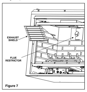
2. Break the Flue Restrictor into two pieces. Do this by bending the part back and forth until it breaks (see Figure 8).
