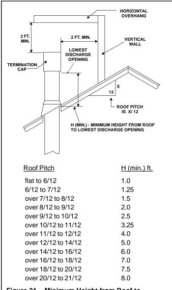
Figure 31. Minimum Height from Roof to Lowest Discharge Opening
