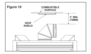
2. Fasten the shield in place using the pilot holes provided in the part. The shield should be oriented such that the 13 1/8 inch dimension (longest dimension) is running in the same direction the elbow is pointing. The shield should be centered directly above the elbow, and positioned so that it creates a 1/2 inch airspace between the shield and the combustible surface. See Figure 20.
