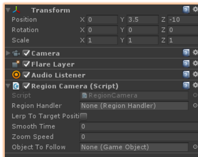
Figure 3 Main Camera with the Region Camera component attached
