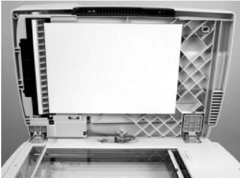
Figure 5-25 Remove the ADF assembly (1 of 3)
