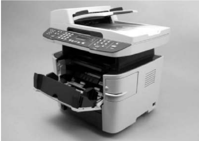
Figure 5-3 Remove the print cartridge (1 of 2)
