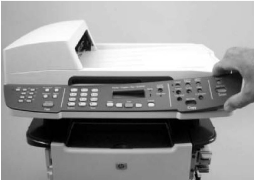
Figure 5-31 Remove the bezel and control panel (1 of 4)
