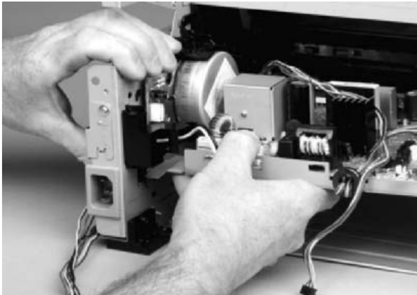
Figure 5-77 Remove the ECU (6 of 8)
