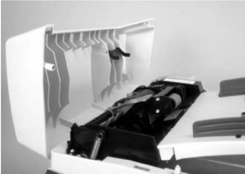
Figure 5-19 Replacing the ADF pickup-roller assembly (1 of 6)
