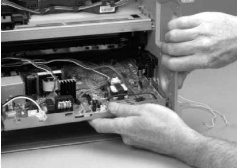
Figure 5-78 Remove the ECU (7 of 8)
