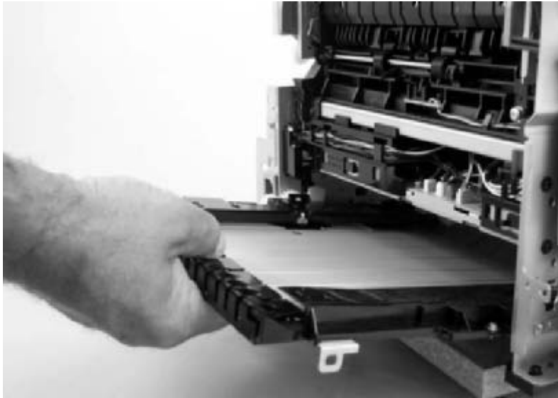
Figure 5-50 Remove the duplex assembly (3 of 3)
