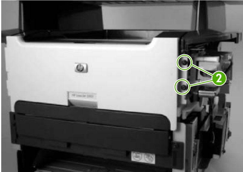
Figure 5-36 Remove the convenience-stapler assembly (2 of 2)
