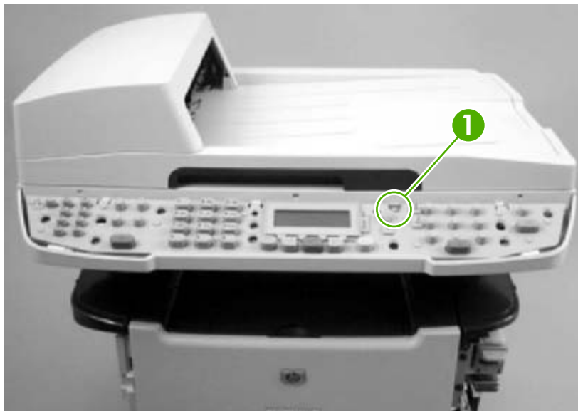
Figure 5-32 Remove the bezel and control panel (2 of 4)
