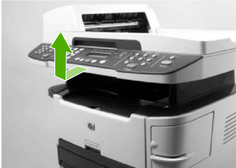
Figure 5-30 Remove the scanner/ADF assembly (3 of 3)
