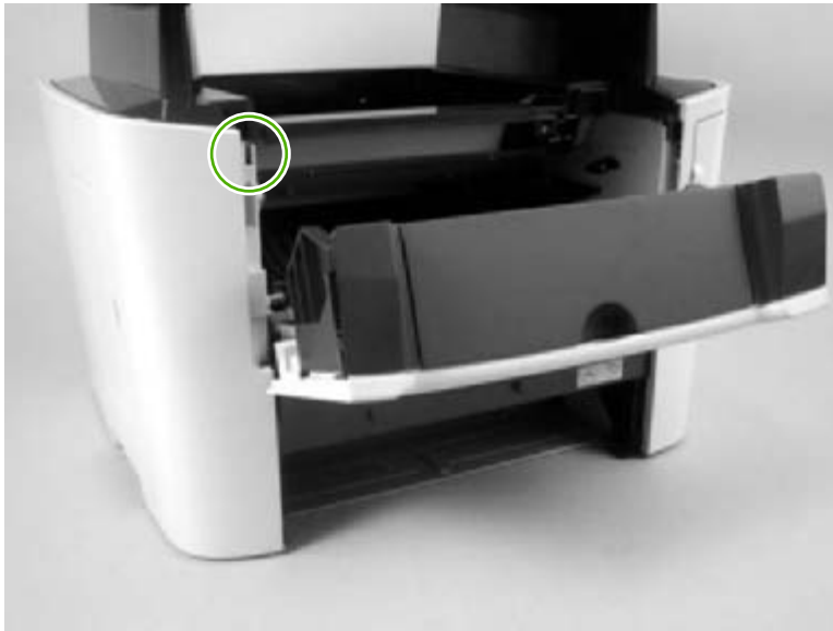
Figure 5-9 Remove the left cover (1 of 3)
