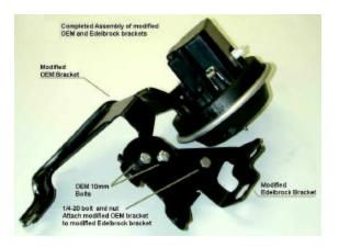
Step 5) Install bracket assembly onto engine. Check for contact between the vacuum actuator boot and the throttle bracket. If contact exists remove more material from the cut line until full clearance is obtained. Tighten all bolts on assembly.
