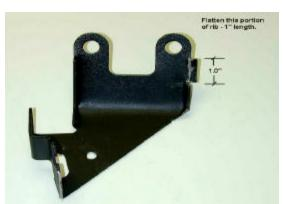
Step 3) The OEM bracket must be cut as shown below. Discard the piece on the right side of the photo.
