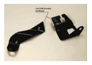
Step 4) Loosely assemble the OEM and Edelbrock brackets as shown below. Some minor adjustments may be required once assembly is bolted on to engine.
