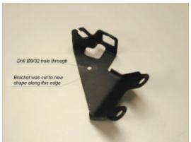
Step 1) Using the guideline on the following page, cut your Edelbrock bracket with hacksaw along specified line and drill Ø9/32 hole.
