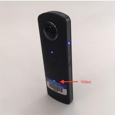
Start recording by pressing the shutter button on the front of the camera. A red light below the video icon will blink while camera is recording. Stop recording by pressing the same button.
