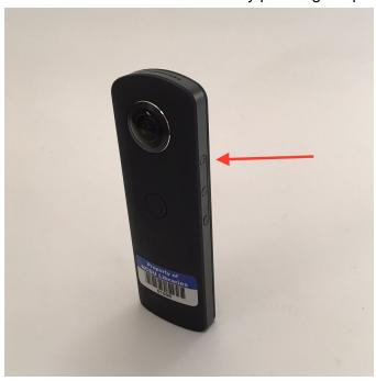
Press the still image/video button on the side to put the camera in video mode. The mode is indicated by the camera or video camera icon on the front.
