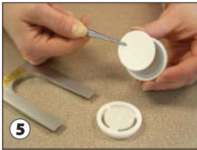
Use the forceps accessory to remove the final collection filter and place it in an appropriate container for shipping to a laboratory.
