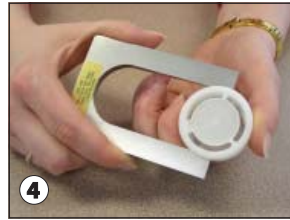
Use the cassette opener accessory to separate the two halves.
