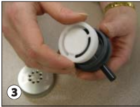
Gently lift filter cassette from exhaust.
