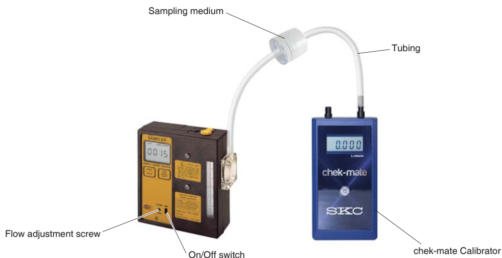
Figure 2. Calibration Train with Filter Cassette
