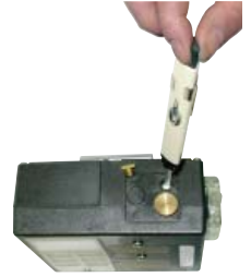
For low flow, turn regulator valve screw counterclockwise.
