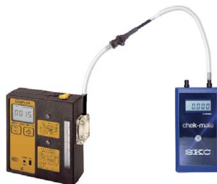
Calibration train with tube in tube holder
