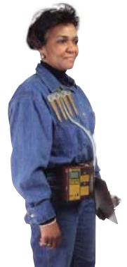
Clip holder to worker and pump to belt.
