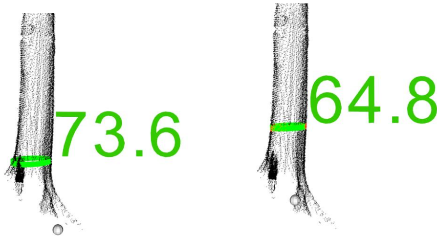
FIG. 3 DIFFERENCES BETWEEN DBH COMPUTED ACCORDING TO THE TREE POSITION NOT ADJUSTED TO TERRAIN LEVEL (LEFT) AND DBH RECOMPUTED WITH TERRAIN CLOUD (RIGHT).
