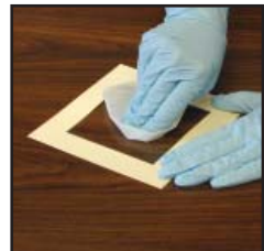
Use a template to specify sample area for samples to be sent to a lab.
