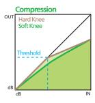
compressor begins to reduce signal levels (attack) and how fast the compressor recovers to a state where it is no longer affecting the input signal (release).
