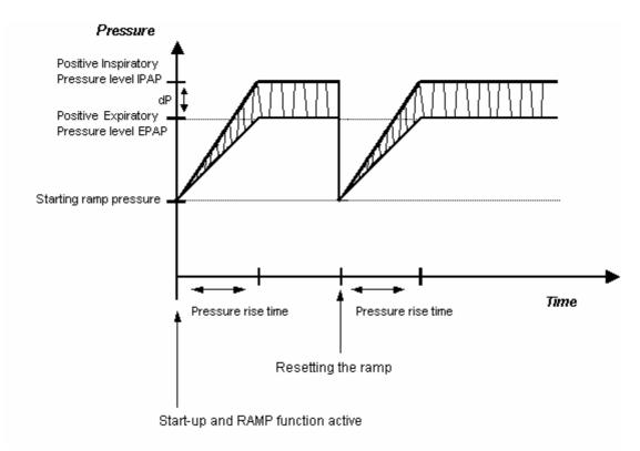
Figure 11 – Pressure Changes and the Ramp Function
