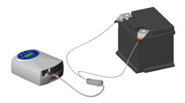
Figure 8 – Connection of the GoodKnight 425 to the battery cable
