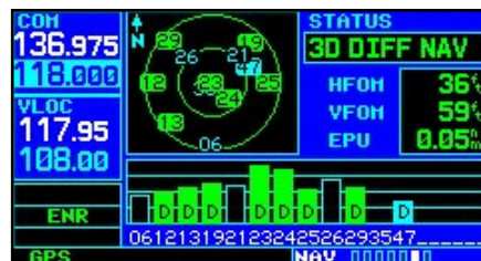
The satellite status page shows the ID numbers for the satellites and the relative signal strength of each satellite received (as a “bar graph” reading).
