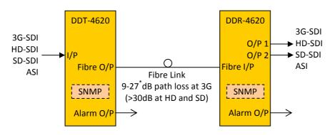
NOTE: \* Fitted with APD detector. 3-18dB when fitted with PIN detector.
