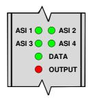
ASI 1, ASI 2 ASI 3 and ASI 4 LEDs correspond to ASI inputs 1, 2, 3 and 4 respectively. When a valid ASI input is present corresponding LED will illuminate green.
