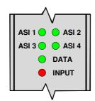
ASI 1, ASI 2 ASI 3 and ASI 4 LEDs correspond to ASI outputs 1, 2, 3 and 4 respectively. When a valid ASI signal is present within the incoming STM-1 signal corresponding LED will illuminate green.
