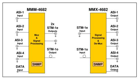
The MMM-4682 and MMX-4682 are part of a family of data transcoders for converting between the commonly used MPEG2 Transport Stream formats for video distribution in the broadcast industry.
