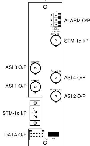
MMX-4682 Rear Assembly Connections
