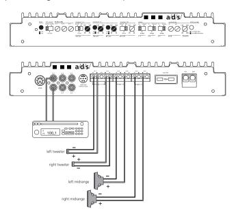
**System 5 -** PH30.2 used in 4-channel mode with high-pass main speakers and low-pass subwoofers. Channels 1 and 2 are configured high-pass for front speakers and channels 3/4, and 5/6 are configured low-pass for bridged output subwoofers. The amplifier is configured for a 4-channel input. Front/rear fade adjusts subwoofer level.
