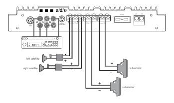
**System 6 -** PH30.2 used in 3-channel bridged mode with two channels dedicated for the main speakers and one bridged channel pair used for a subwoofer. Channels 1/2, and 3/4 are configured high-pass for the main front speakers using a single pair of RCA inputs to produce a bridged mono output.
