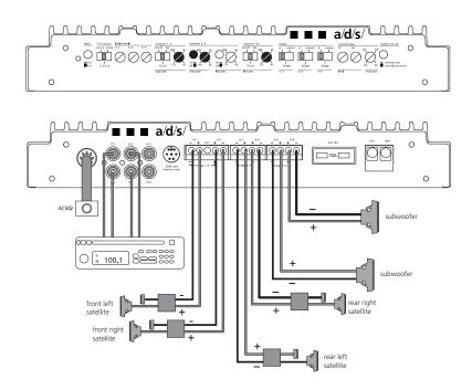
**System 2 -** PH30.2 used in 5-channel mode with the AC502 providing level control for bridged channels 5 and 6. 1 and 2 are high-passed for front speaker and channels 3 and 4 are high-passed for rear speakers. Although shown as a 4-channel input, the source unit can be either 2 or 4-channel depending on the setting of the 2/4 channel switch.
