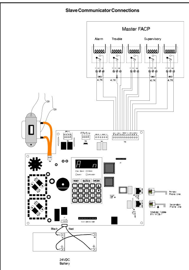
Relays in Master FACP activate various input circuits on the slave communicator. Messages (event codes) programmed for a particular input circuit (channel) will be transmitted to the central station upon relay activation.
