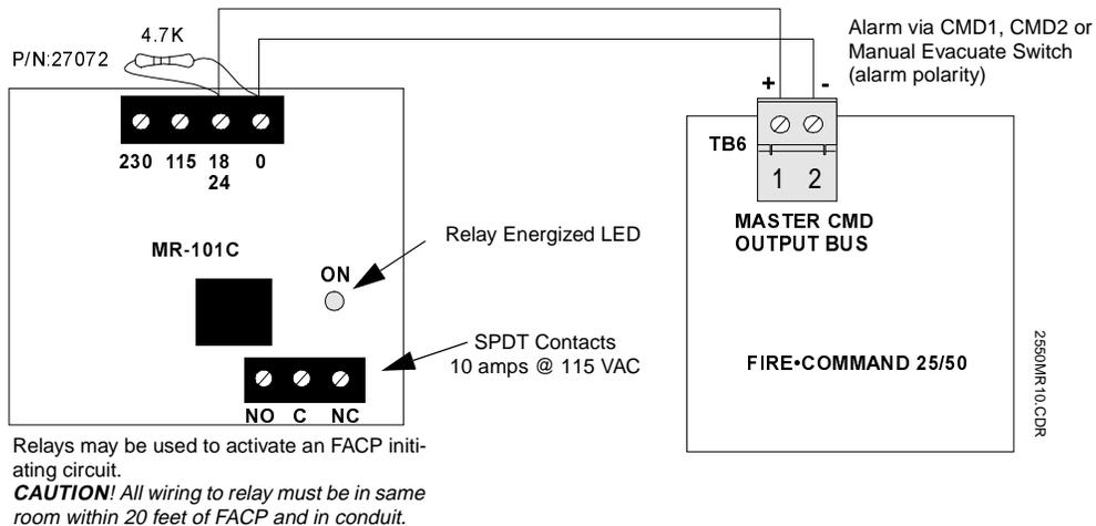
The MR-101C (one Form-C relay) and MR-201C (two Form-C relays), which are manufactured by Air Products and Controls, include an enclosure.
