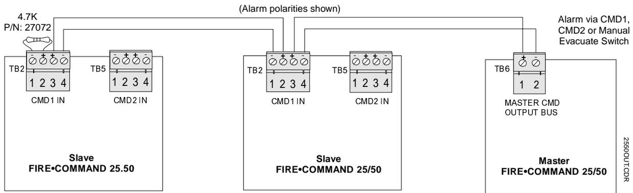
The maximum line resistance from the main VECP to the last VECP is 130 ohms (65 ohms per conductor).
