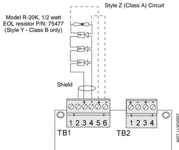
Shielded cable is not required, however, shielded cable will reduce RFI/EMI emissions and susceptibility. For additional information, refer to Appendix E.
