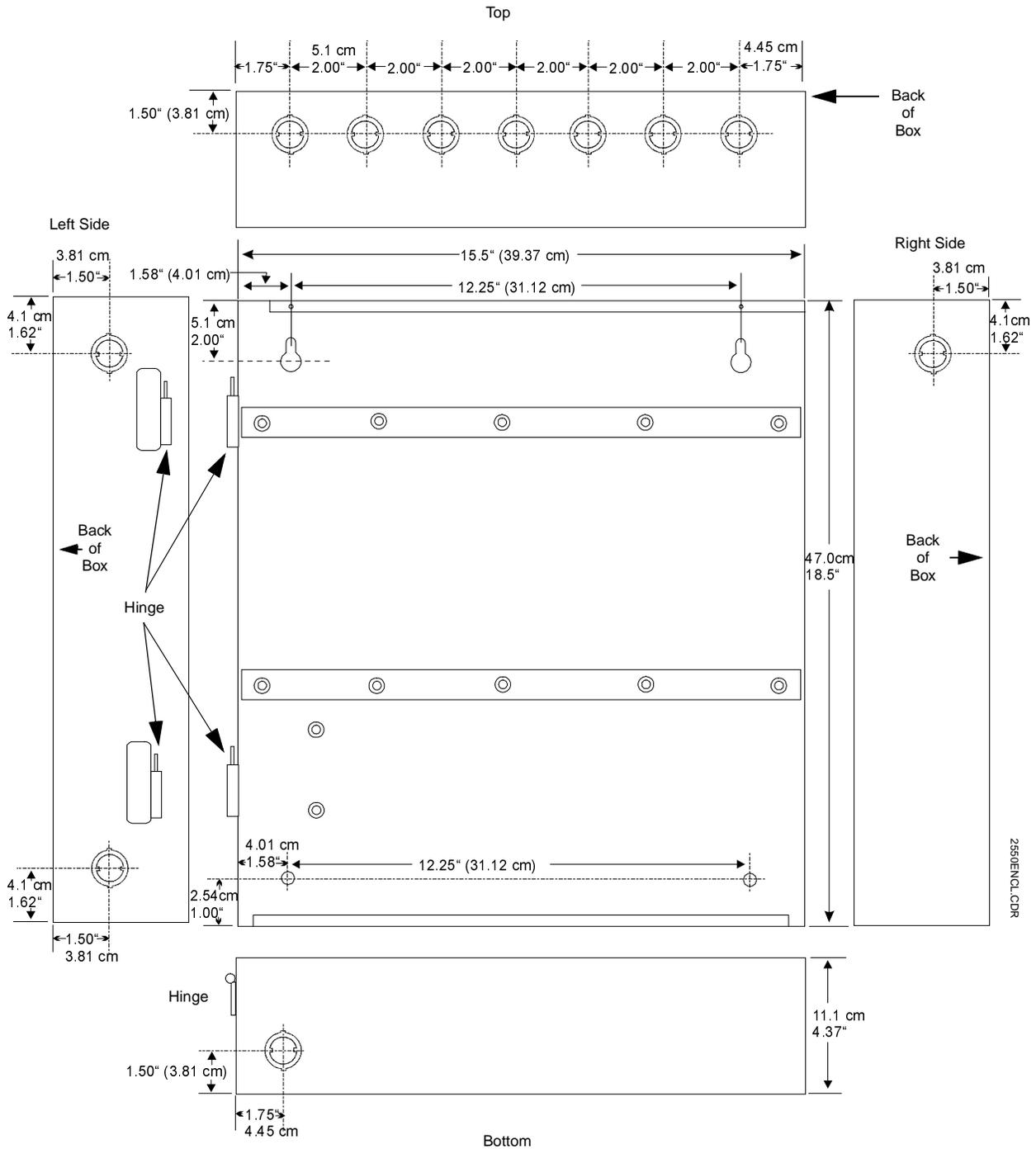
FIGURE 3-4:VECP Backbox and Battery Box
