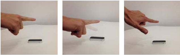
Figure 1. The mid-air gestures (from left-right: single finger cursor control, screen tap, thumb trigger)
