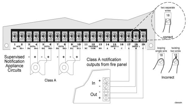
Figure 4-4 Class A Supervised Input/Output Connections
