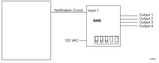
Figure 6-1 Input 1 Activates All Four Outputs
