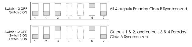
Figure 4-10 Faraday Synchronization Configurations
