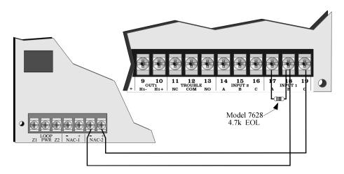
Figure 5-5 Connection to the SK-2224 Fire Alarm Control Panel
