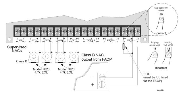
Figure 4-5 Class B Supervised Input/Output Connections
