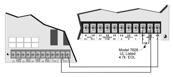
Figure 5-6 Connection to the SK-4224 Fire Alarm Control Panel
