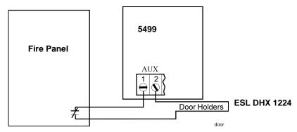
Figure 6-7 Door Holder Wiring Example
