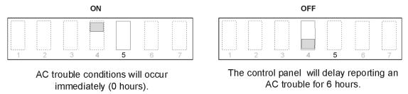
Figure 4-15 Setting DIP Switch 4
