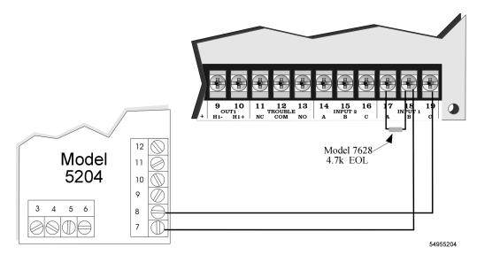
Figure 5-3 Connection to 5204 Fire Control/Communicator
