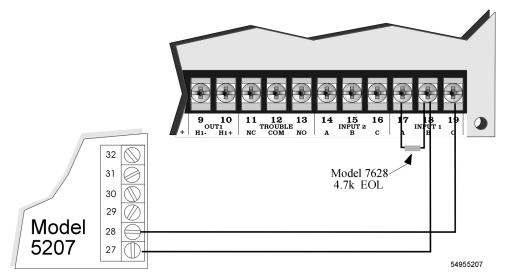
Figure 5-4 Connection to 5207 Fire Control/Communicator
