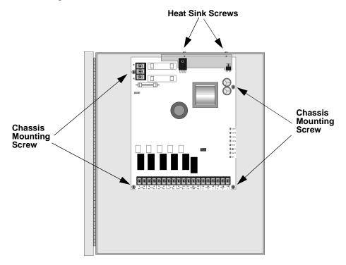
Figure 7-1 Mounting Screw Locations
