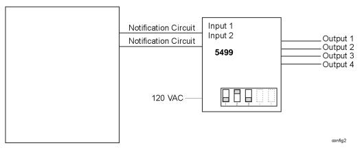
Figure 6-2 Input 1 Activates Outputs 1 and 2; Input 2 Activates Outputs 3 and 4
