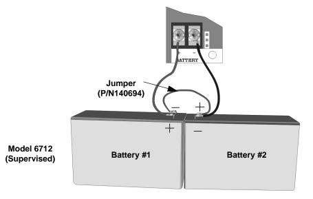
Figure 4-7 Battery Connection
