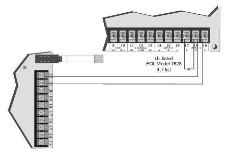
Figure 5-2 Connection to 5104B Fire Communicator
