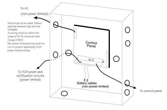
Figure 4-1 Sample Wire Routing
