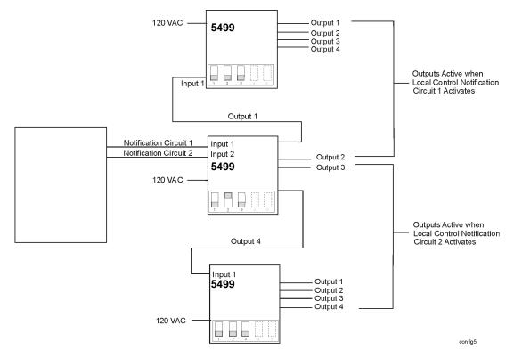
Figure 6-5 Each Control Activates Five Notification Appliance Circuits
