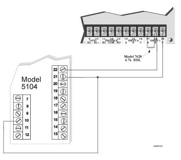
Figure 5-1 Connection to 5104 Fire Communicator
