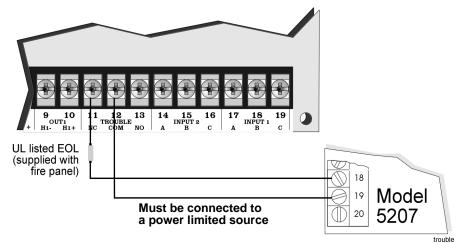
Figure 4-3 Trouble Relay Connection Example
