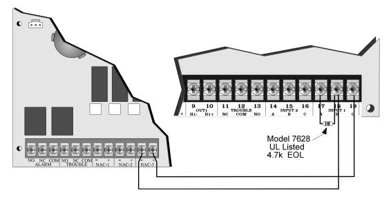
Figure 5-7 Connection to the SK-6324 Fire Alarm Control Panel
