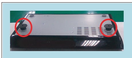
[Fig. 3] Attach rubber to the lower part of Media-Box.
