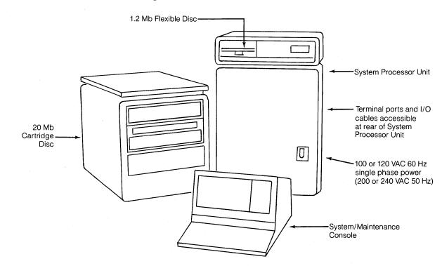
Note: Power outlets for disc and terminal not provided in System Processor Unit. Under certain power line conditions at the system site, an isolation transformer or other line conditioning equipment may be required. Refer to Site Preparation section of this guide.
