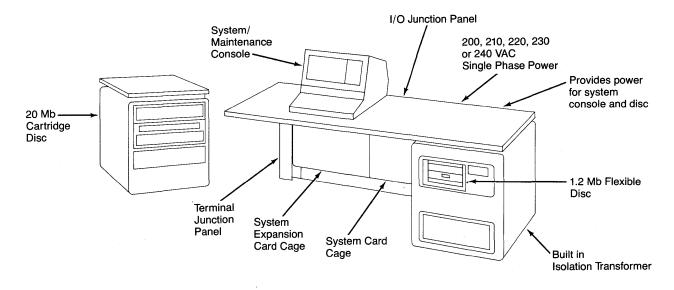
Note: Under certain power line conditions at the system site, an isolation transformer or other line conditioning equipment may be required for add-on disc and magnetic tape drives.
