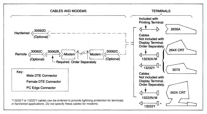
MTS/3000 Hardwired Data Link (Asynchronous Cable Configurations)
