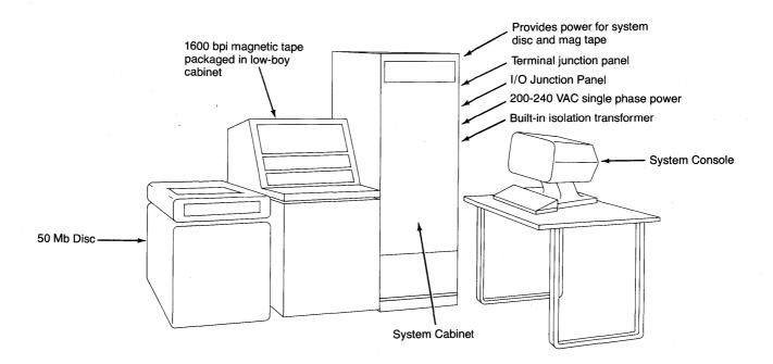
Note: Under certain power line conditions at the system site, an isolation transformer or other line conditioning equipment may be required for add-on disc and magnetic tape drives.
