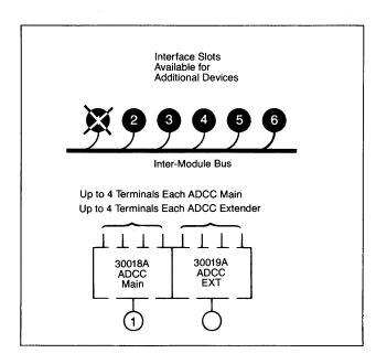
As a result, the options that have been chosen and the interface slots they occupy will be evident at a glance. DO NOT EXCEED THE TOTAL NUMBER OF AVAILABLE INTERFACE SLOTS ON THE INTER-MODULE BUS.
