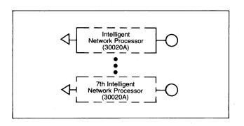
Connecting Additional Devices. Spare interface slots (numbered "circles") connected to the IMB are available for additional devices and can be interfaced to either Asynchronous Data Communication Controllers (ADCCs), General I/O Channels (GICs) or Intelligent Network Processors (INPs).
