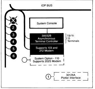
As a result, the options that have been chosen and the interface slots they occupy will be evident at a glance. DO NOT EXCEED THE TOTAL NUMBER OF AVAILABLE INTERFACE SLOTS ON THE IOP BUS.
