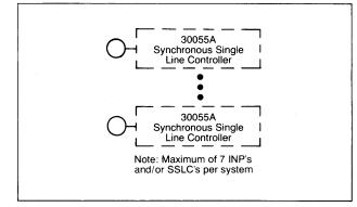
Interfacing Optional Equipment Through Interface Slots. Spare interface slots (numbered "circles" connected to the IOP Bus) are available for additional products, and can be occupied by optional equipment identified with an attached "circle."
