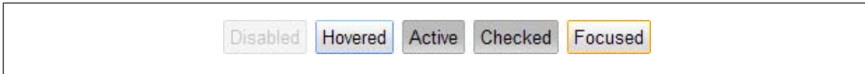
Figure 8-10. goog.ui.CustomButton rendered in various states using the CSS defined in custombutton.css . The Active and Checked buttons intentionally have the same CSS so that a button that is actively pressed down appears the same as a toggle button in the checked state.
