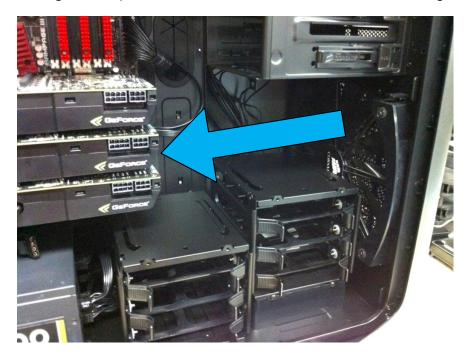
This reconfiguration allows for direct airflow from the front intake fan to reach the graphics cards for superior cooling performance. It's also possible to remove the lower drive cage, as seen here.
