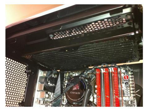
Depending on the motherboard components and clearance issues, in some cases the fans should be installed outside the case, as shown below. There is sufficient clearance beneath the top filter exhaust for this.
