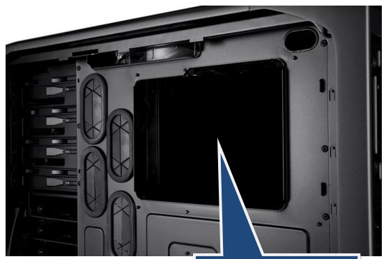
The CPU backplate cutout provides the user with an easy way to install an aftermarket heatsink that utilizes a custom backplate for mounting.
